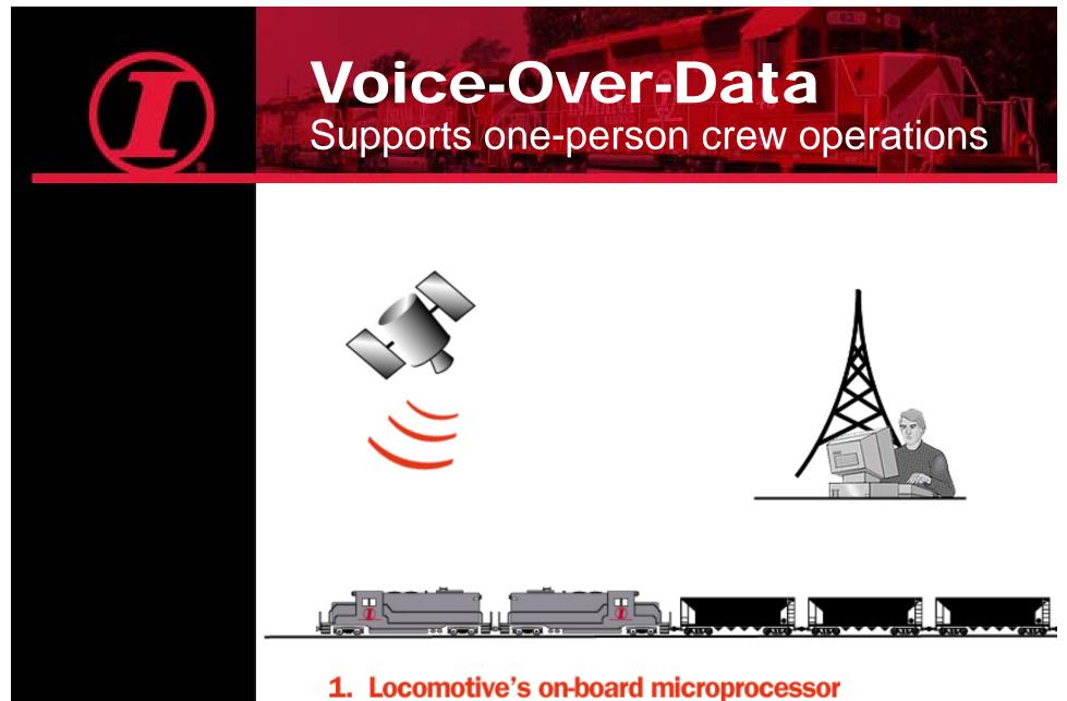
1. Locomotive's on-board microprocessor receives signals from GPS satellites.
