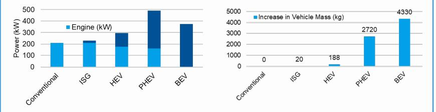
Note: Autonomie class 8 truck weights correlate well with results from electric drive implementation on class 8 trucks by TransPower.
