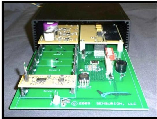
*Sensurion's RSU – (Remote Sensor Unit), configured for manned vehicle or building application*
