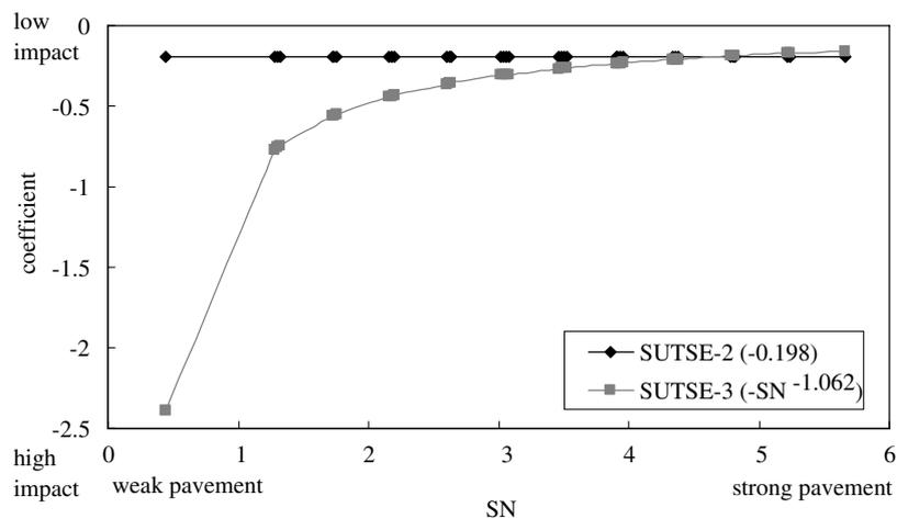
Fig. 2. Effect of non-linear structural number component.
