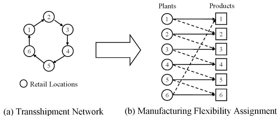
Figure 3: Transshipment unidirectional chain and manufacturing chain assignment networks
